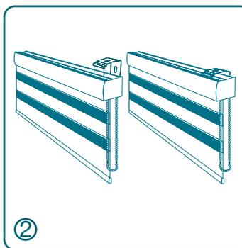
1. Install brackets firmly into place, use raw plugs where necessary to ensure brackets are securely fitted.
